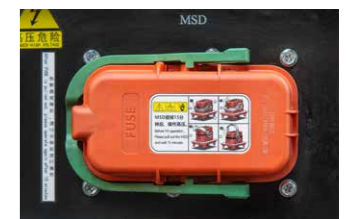
The MSD maintenance switch
